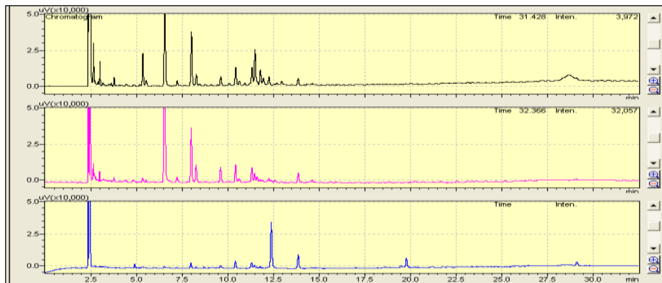
Figure 6. GC Analysis of Lipid Composition from Culture GN/PA/N4 Grown in 5L Lab-Scale Fermentation.
