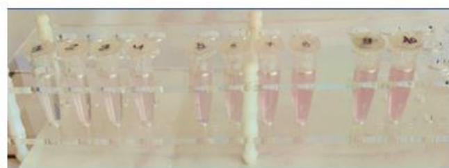
Figure 3. Color reaction with o-toluidine for glucose concentration determination.
