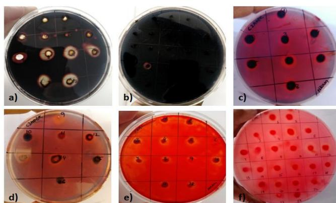
**Figure 4.** Amylase and cellulase production exhibited by culture filtrates of fungal endophytic isolates. (a-b) amyolytic activity, indicated by clear zone around the well over starch agar plate stained by Iodine solution (c-f) cellulolytic activity, indicated by pale yellow halo around well on carboxymethyl cellulose agar, stained in aqueous Congo red.
